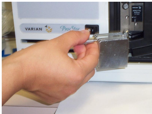
Figure 32 Visible lamp housing removed
