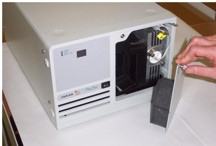
Figure 24 Removing the front ProStar 325 panel
