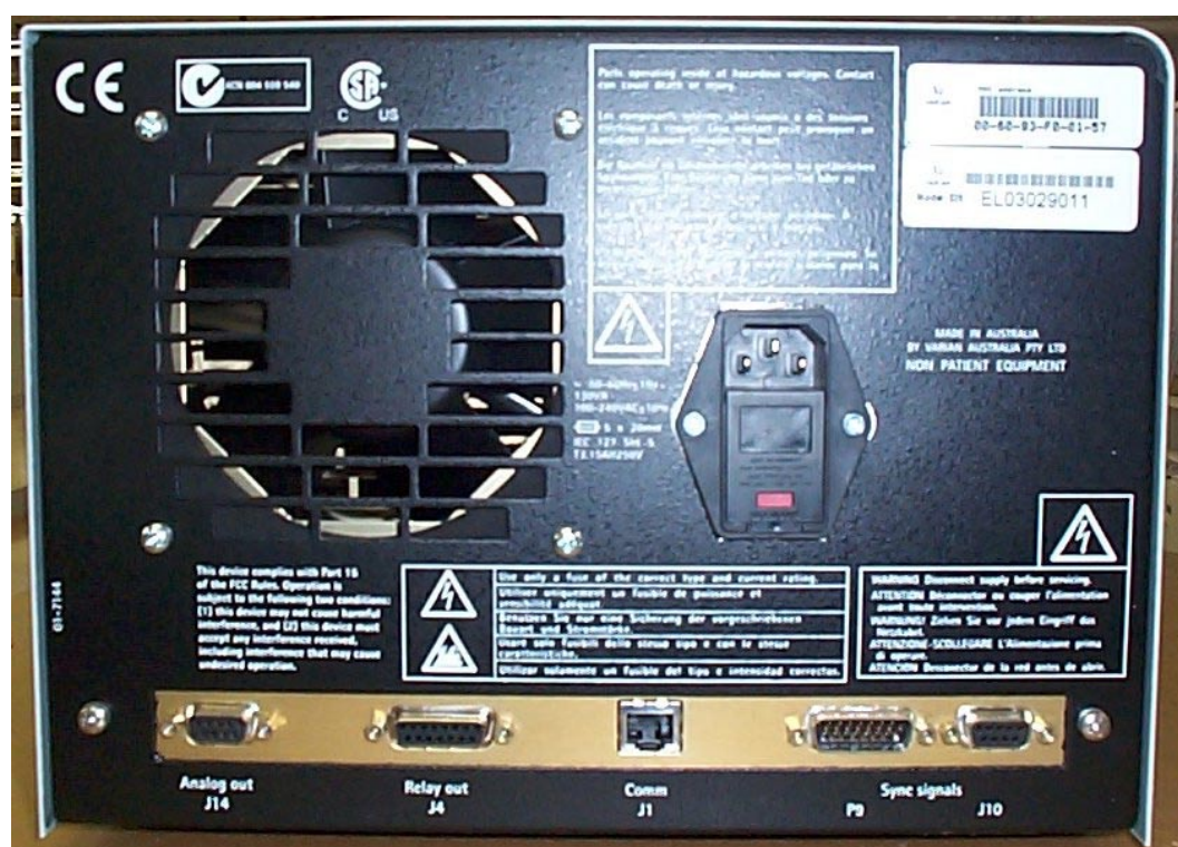
Figure 2 ProStar 325 rear panel services
