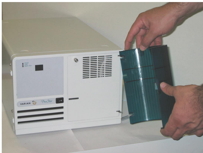
Figure 15 Installing the ProStar 325 door
