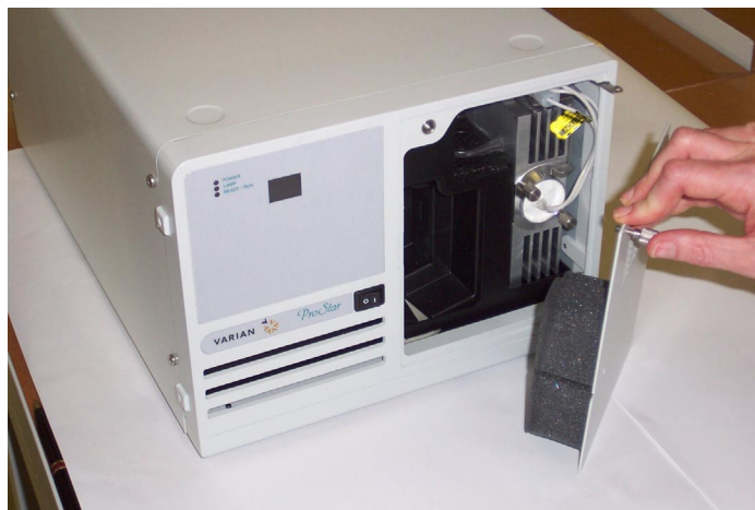
Figure 12 Removing the front panel from the ProStar 325
