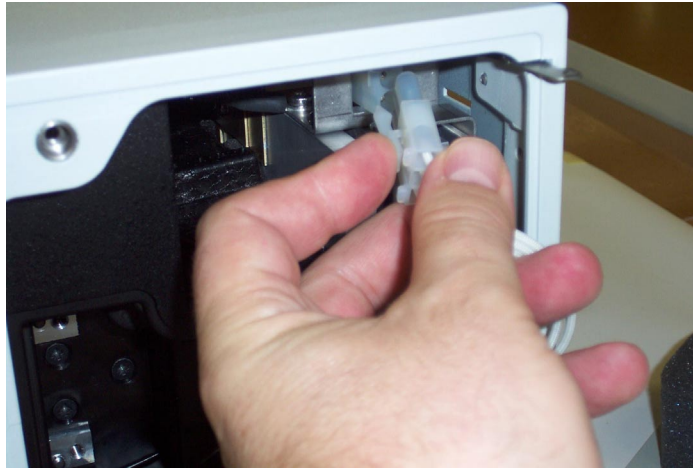
Figure 25 Removing the lamp 3-way connector
