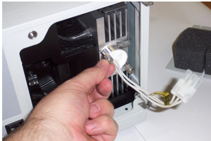
Figure 28 Undoing the second lamp screw
