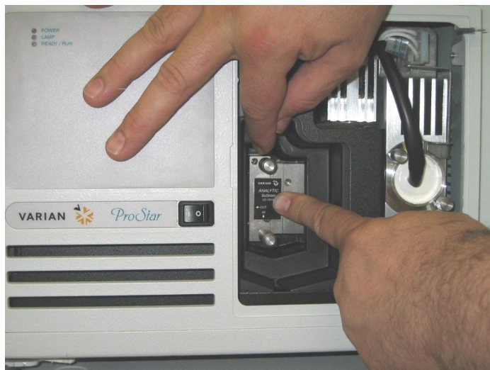
Figure 13 Positioning the flowcell in the flowcell compartment
