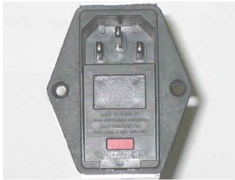
Figure 33 Mains input connector and fuse compartment
