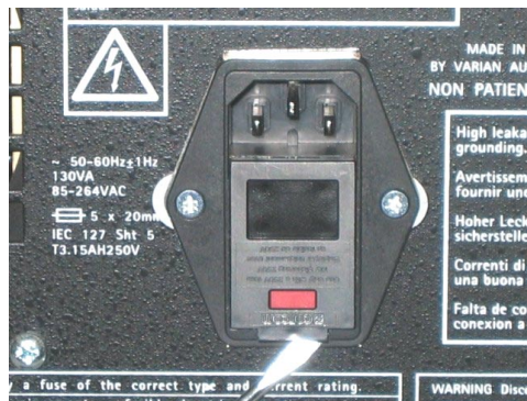
Figure 34 Lifting the fuse compartment cap
