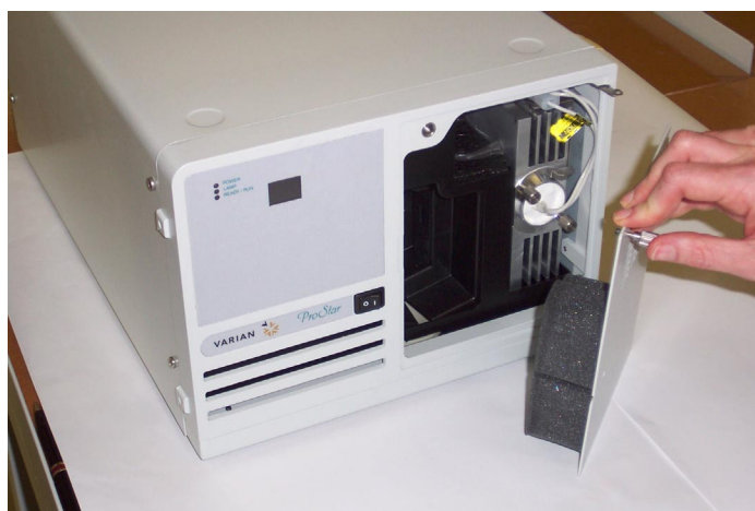
Figure 30 Removing the ProStar 325 front panel
