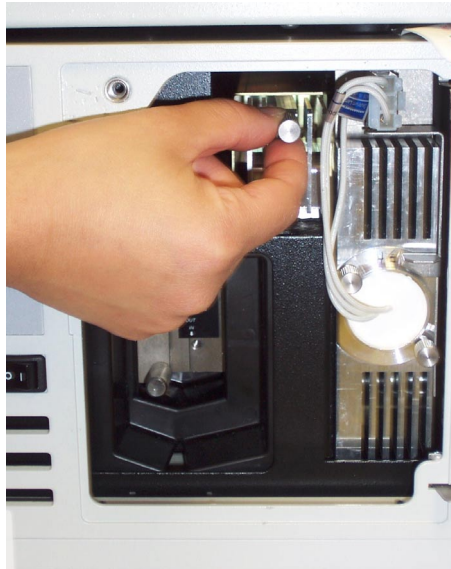
Figure 31 Undoing the visible lamp screw
